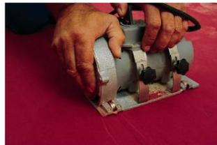
The melting wire is applied with an automatic welding machine or a hand torch with an instant welding nozzle or a polyolefin nozzle 5 mm in diameter. The rear part of the foot (air outlet) of the instant welding nozzle should not be broader than the milled groove (3.5 mm). We recommend automatic welding machines in which the melting wire runs without tension, the temperature is controlled constantly and the welding rod is put into the milled groove without pressure.
